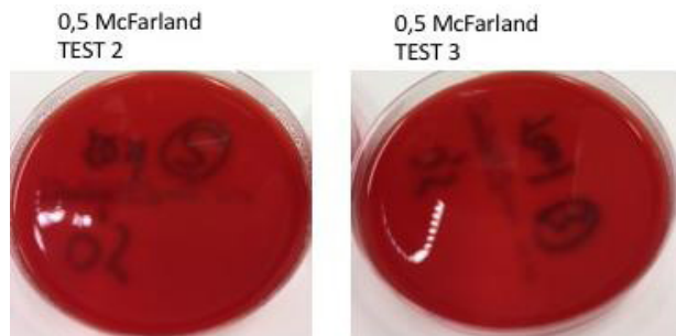
Figure 3: Two additional blood agar plates, each with 0.5 McFarland of the micrococcus suspension, were placed in two different areas of the room with indirect UVC radiation (shadow areas). None of the plates showed any bacterial growth.
